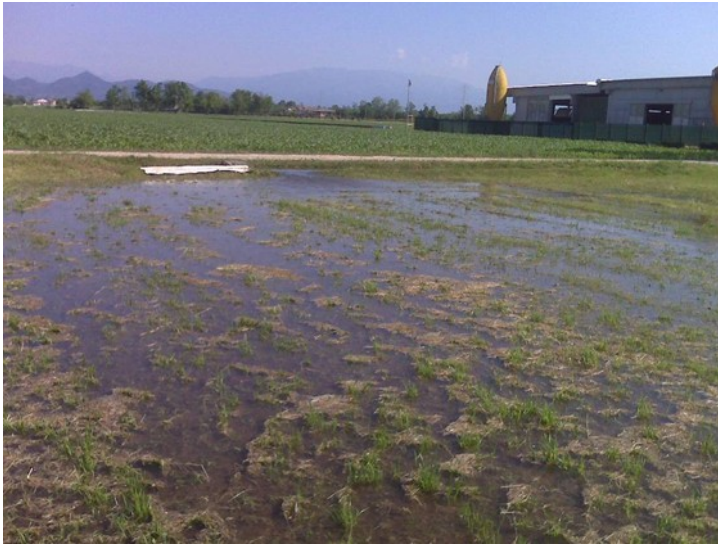
FIGURE 7 – Right: The test field and the progressive water distribution during the initial phases of water provision in Busta site (TV); Top: Photograph of the MAR test carried out by Piave Irrigation Consortium
