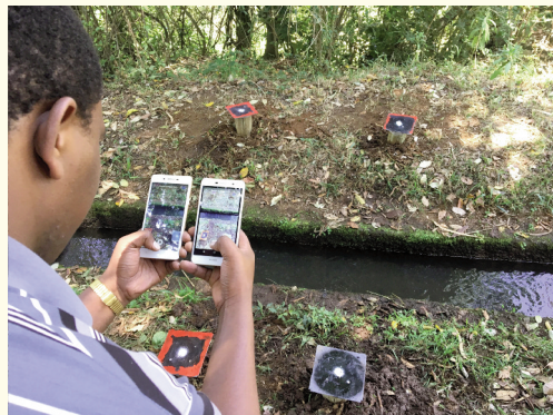
Figure 12: Measuring discharge of a small irrigation canal with 2 different smartphones in Tanzania for comparison.
